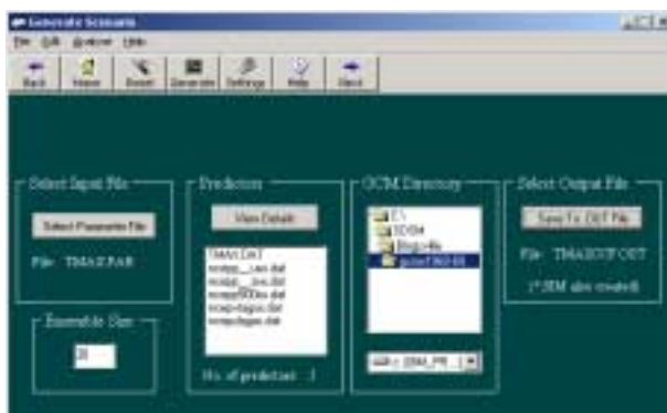
Figure 11.1 The Generate Scenario screen, showing selections for the Blogsville example using GCMX predictors representing the current (1960–1989) climate.
